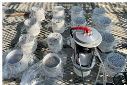
Fig 1. Experimental setup, including gas flux analyzer.
