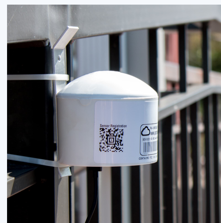
Fig. 1: PurpleAir PA-II particulate sensor zip tied to a fence
